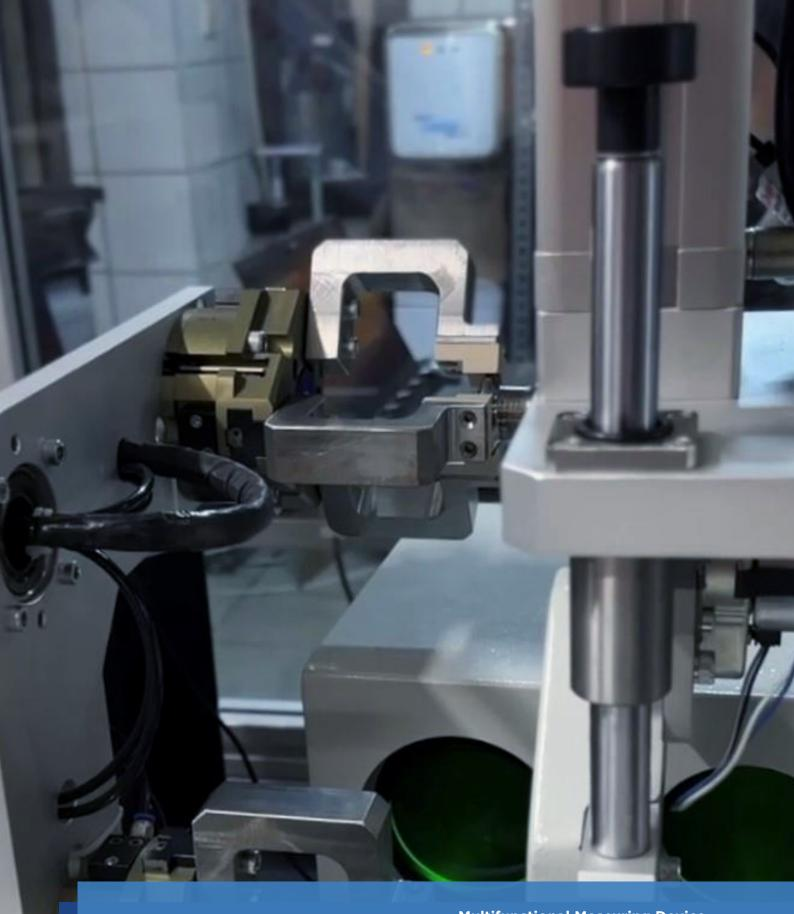
**Multifunctional Measuring Device** According to customer demand, elements such as diameter, length, circularity on a cylindrical part are measured with cameras by rotating the part
