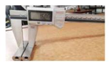
**Special Cylinder Jaw Caliper** Specially designed for the customer, this cylinder jaw caliper is used for tire surface width measurement on rims.
