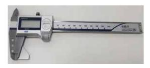
**Special Cylinder Jaw Caliper** Example of caliper with specially prepared jaws for customer special measurement demands on wind vane blades.
